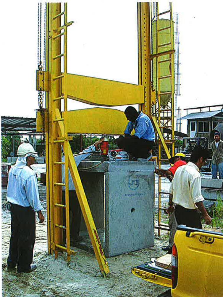
Load Testing of R.C. Box Culverts
